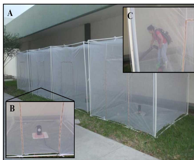
Figure 3A. Experimental cages in semi-field trials. B. Traps were isolated to avoid damage by predators. C. Mosquitoes extraction was carried out with the backpack aspirator
